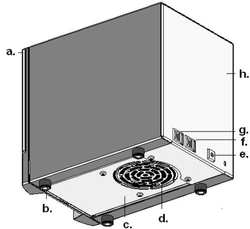
2. Connect the Ethernet cable to port 0 (f.).
